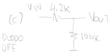
$$\frac{V_{out}}{V_{in}} = \frac{100}{100 + 4.2} = 0.96$$
