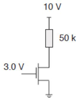
**R:  $V_{DS}=0.56\text{ V}$  e  $I_{DS}=0.18\text{ mA}$**
