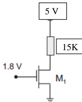
**R:  $V_{DS}=0.53\text{ V}$  e  $I_{DS}=298\text{ uA}$**
