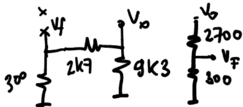
$$V_F = V_0 \frac{300}{300} \therefore \beta = \frac{V_F}{V_0} = 0.1 \quad \text{Logo } A_V \approx \frac{1}{\beta} = 10$$
