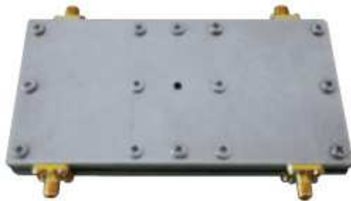
9. The prototype coupler was fabricated on RT/duroid 5880.
