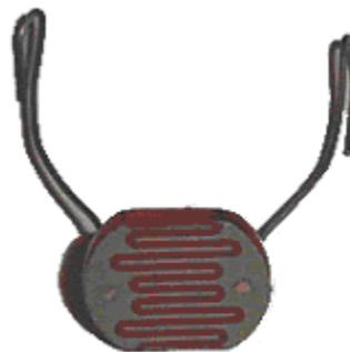
**Figura 1.** LDR (Light Dependent Resistor).
