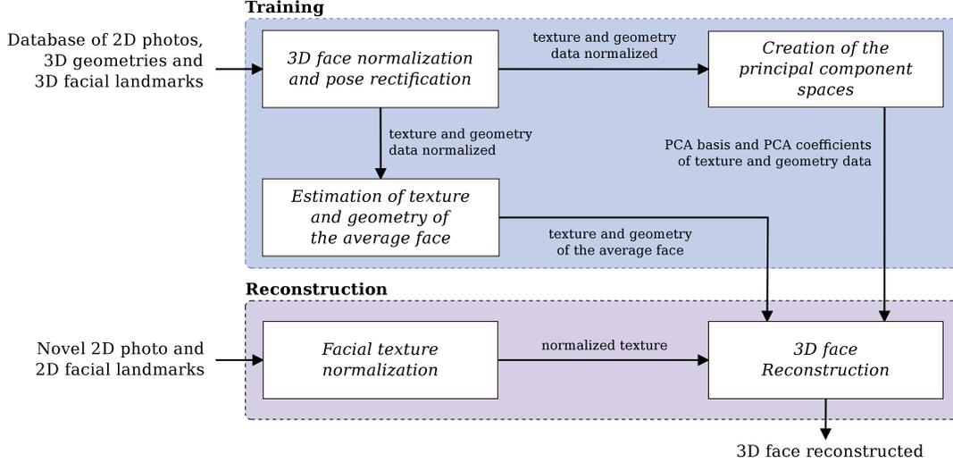
Figure 2. Schematic data flow diagram of the 3D facial reconstruction system (dotted lines). Each block (solid lines) represents a process, while each arrow represents the information flow between processes.
