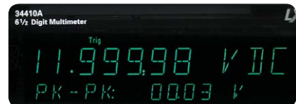
Figure 3. An example of a DMM that can display both DC and AC voltage measurements simultaneously
