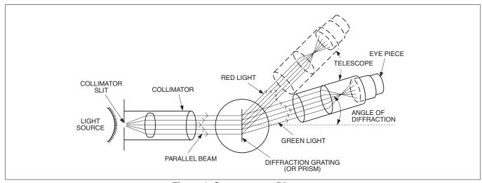
Figure 1 Spectrometer Diagram
