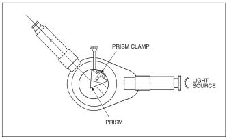
Figure 10 Mounting the Prism
