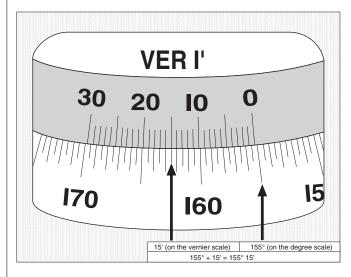
Figure 6 Reading the Vernier Scales
