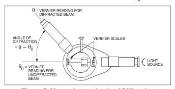
Figure 5 Measuring an Angle of Diffraction
