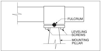
Figure 4 Leveling the Telescope and Collimator
