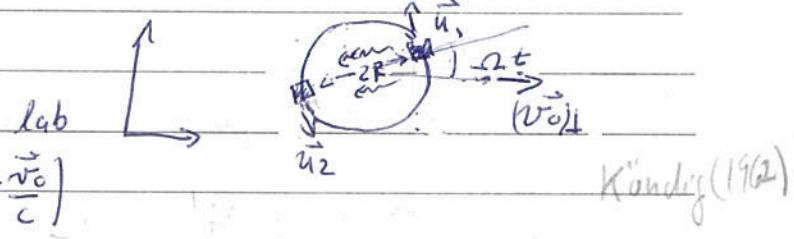
$$\text{de (11): } \frac{\omega_1 - \omega_0}{\omega_0} = \left( \frac{\vec{u}_1 \cdot \vec{v}_0}{c} \right) \cdot \left( \hat{m} + \frac{\vec{v}_0}{c} \right)$$
