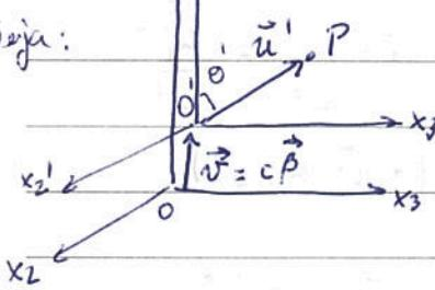
$$\left\{ \begin{array}{l} dx_0 = p_v (dx_0' + \beta dx_1') \\ dx_1 = p_v (dx_1' + \beta dx_0') \\ dx_2 = dx_2', \quad dx_3 = dx_3' \end{array} \right.$$
