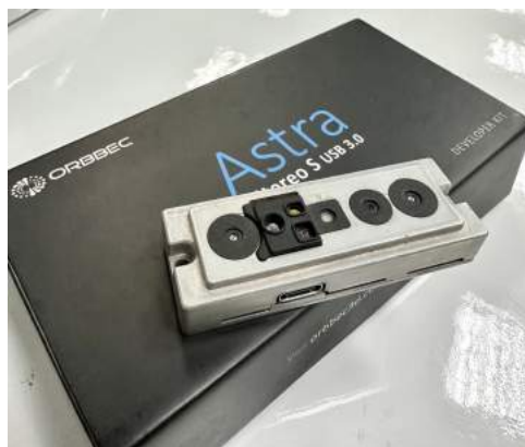
Figura 3.3 – Sensor ASTRA STEREO S U3
