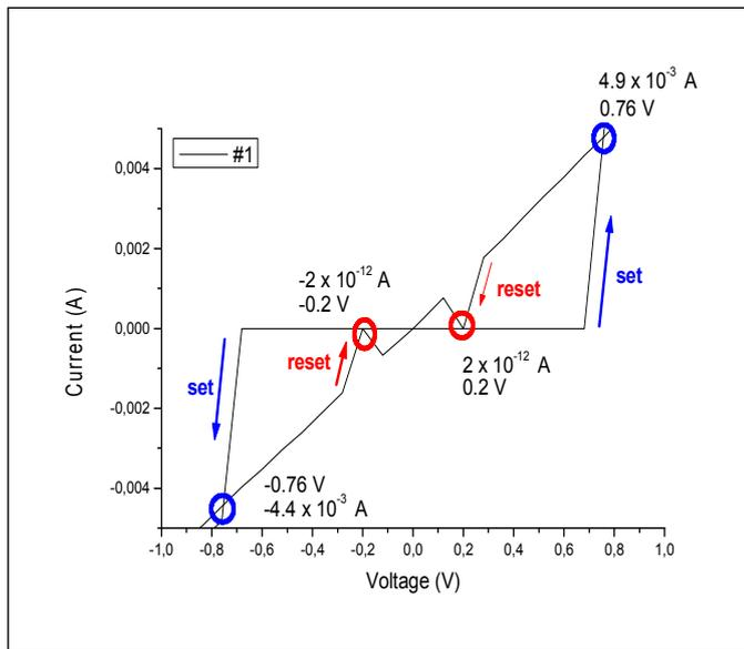
Fig. 4. Typical I-V curves of ITO/CuO/GO+1%Cu/CuO/Al structure.
