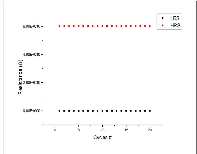
Fig. 2. Initial endurance test for ReRAM structure.
