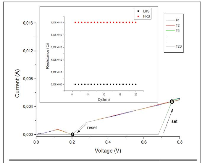
Fig. 5. I-V characteristics of ITO/CuO/GO+1%Cu/CuO/Al. The upper left inset is high resistance state and low resistance state depending on the switching cycle.
