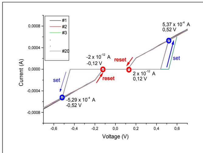
Fig. 1. I-V characteristics of ITO/GO+1%Cu/Al.
