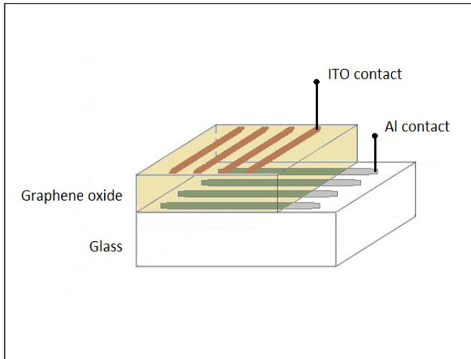
Fig. 6. Resistive random access memories array architecture.
