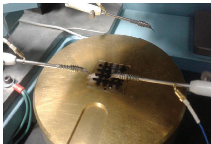
Fig. 2. Arrangement of the device connected through microprobes.
