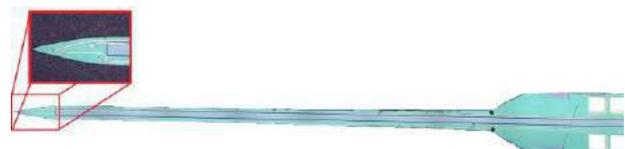
Fig. 2. A SiC optrode developed at USF [14]. The optrode features four platinum recording electrodes and an amorphous SiC coated SU-8 waveguide. The electrodes are desigeld to be connected to a neural signaling amplifier at the pads on the right side of the image.
