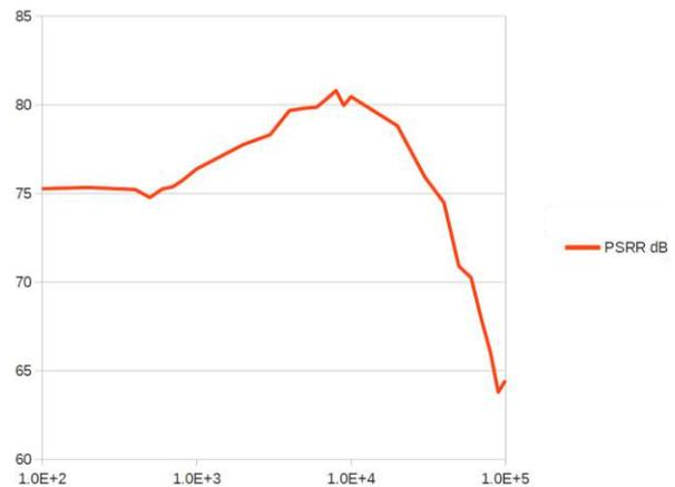
Fig. 8. Measured power supply rejection rate (PSRR) vs frequency – displaying a worst case value of 64dB.
