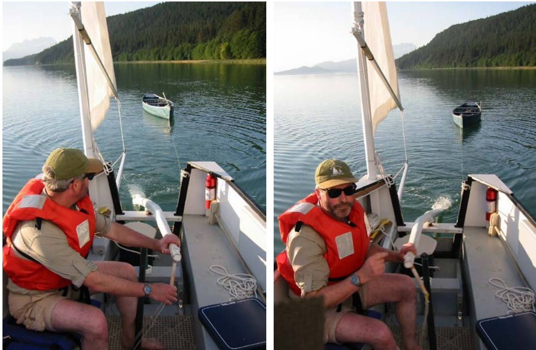
Figure 2 – Modern boat propelled by sculling a western version of Ro.
