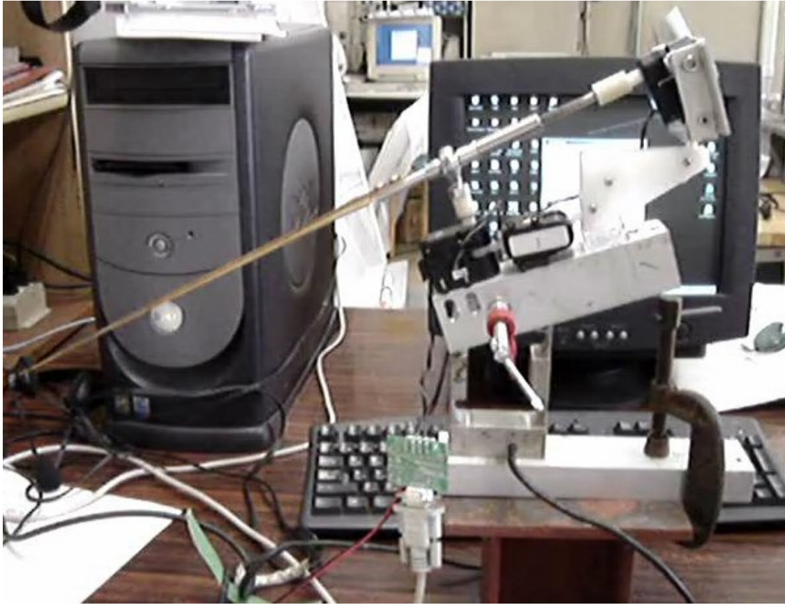
Figure 11 – Sensor assembly used to calibrate the simulation. The Ro-bot mechanism was first mounted over a thrust block, where the impulse produced in the Y-direction could be recorded.
